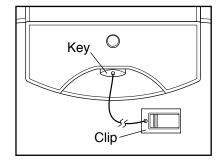
sole. Test the clip by carefully taking a few steps backward until the key is pulled from the console. If the key is not pulled from the console, adjust the position of the clip as needed. Follow the steps below to operate the console.
